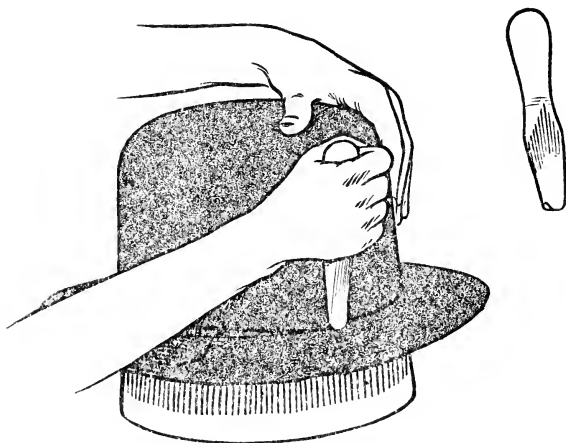
THE CORD IS WORKED DOWN TO THE BAND-MARK WITH THE RUNNER-DOWN
